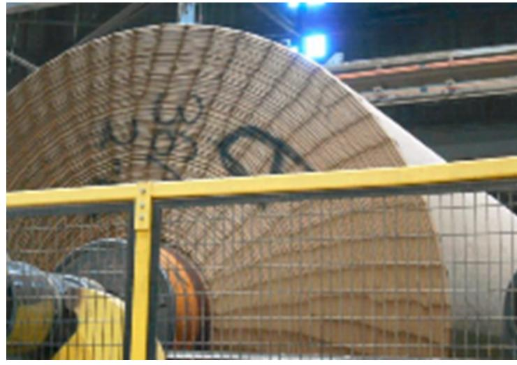
This causes spool losses, winder runnability losses, sheet breaks
